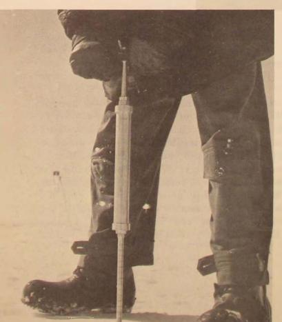
The "weasel" (above) was the main vehicle for overland transportation during "Mint Julep" research. An outgrowth of the World War II T-15 oversnow tractor, the weasel replaces the traditional dog team and sled. The penetrometer (left) is a special instrument to test the physical characteristics of the ice and snow near the camp site. Natural landing fields exist where basal glacial ice is exposed or is covered by a thin film of refrozen melt-water ice.
